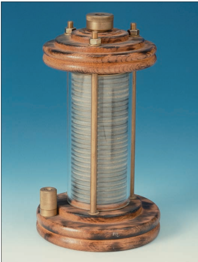
The “Ritterian Pile”, developed by Ritter in 1802, is considered to be the forerunner of the accumulator.
